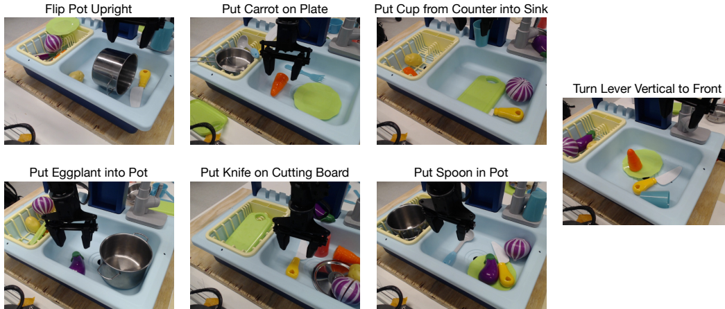
Figure 7: Original BridgeData V2 sink environment tasks. Images from sample demonstrations in the sink environment from the original BridgeData V2 dataset reveal that all demonstrations in this environment were initialized such that the robot’s end-effector was positioned immediately above the target object. Note that these initial states are different from the initial states we use in our BridgeData V2 evaluation tasks shown in Fig. 6. In our evaluations, we always initialize the robot’s end-effector to a fixed location above the sink, rather than positioning it directly above the target object (except for one task: “Put Eggplant into Pot (Easy Version)”).
